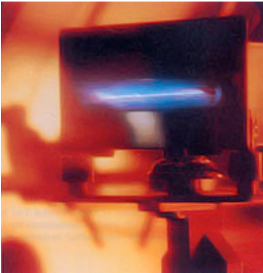
Intense ion beams gen-er-ated by FEEP thrust-ers (cour-tesy ESA)
